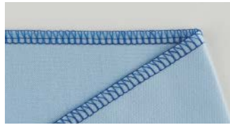
4-Thread Overlock Uses 2 needles and 4 threads to securely sew together knitted fabrics.
